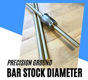
Precision ground bar diameter tolerance -0.0005"-0" required. Straightness Tolerance 0.01" per ft. suggested
